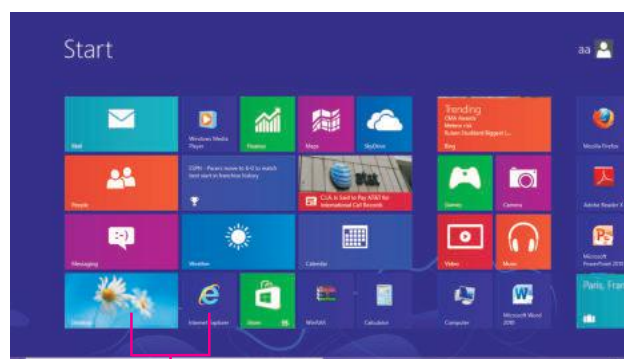
Left scroll arrow Tiles Scroll bar Right scroll arrow Zoom icon Windows 8 Start screen
