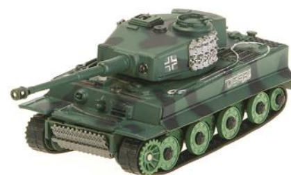
tanks have broad chains that increase the area of contact
