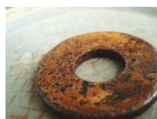
Rusting of iron
